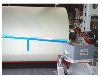
For easy alignment we recommend the optional mounting angle MF330flex.
