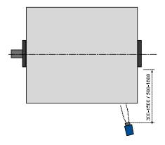
The sensor gets placed in a distance of min. 300 mm from the biggest tambour diameter.
